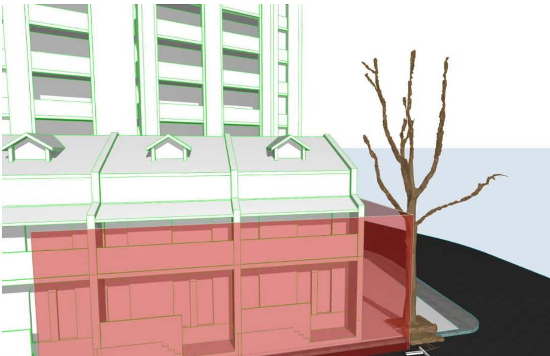
Figure 14 – View of 3D computer model of building and data obtained for trees stripped down to the major branches for T06. Red line/zone indicates scaffold cut line. Note that the majority of main branches are well clear of proposed building and should not require any pruning. (Image Source: Arterra)
